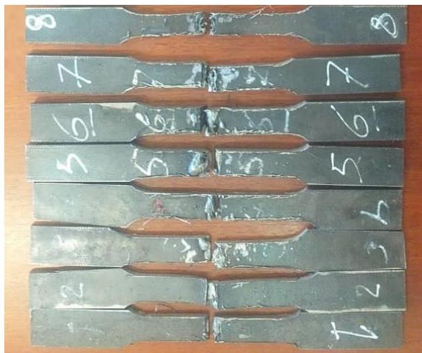
Figure 4: Samples used for tensile strength
