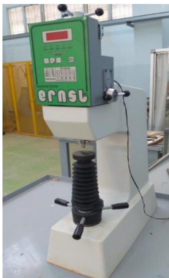
Figure 5: Ernst Rockwell hardness tester
