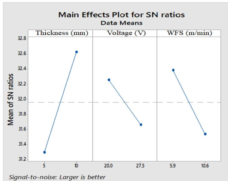
Figure 2. Main effect plot for S/N ratio for the welding factors
