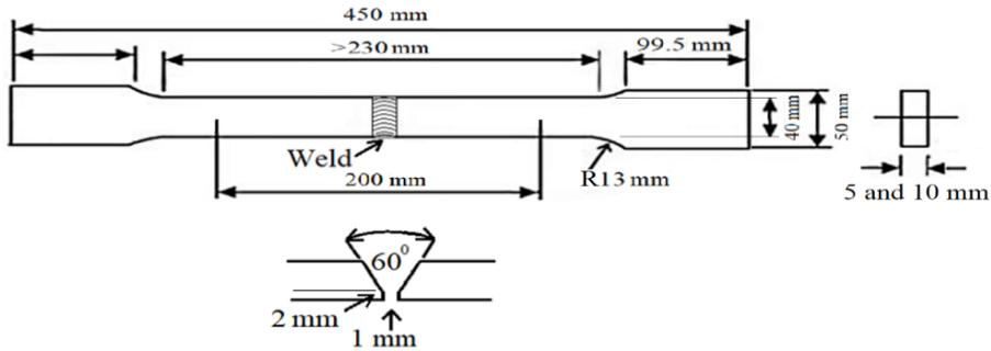
Figure 1. Samples dimensions for tensile test made according to ASTM E8/E8M (ASTM, 2021)
