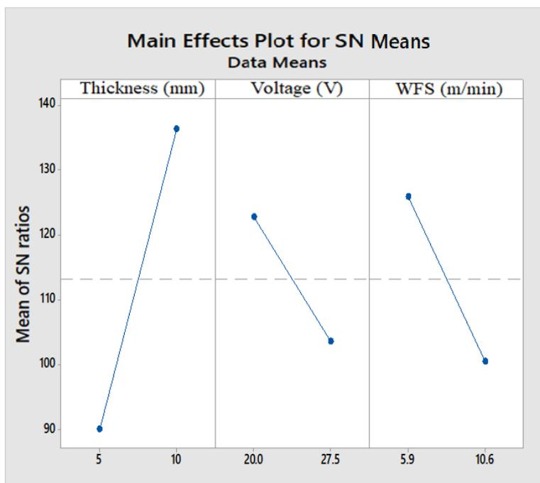
Figure 3. Main effect plot for means for the welding factors
